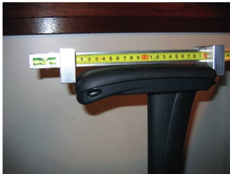
Figure 59 — Armrest length callipers
